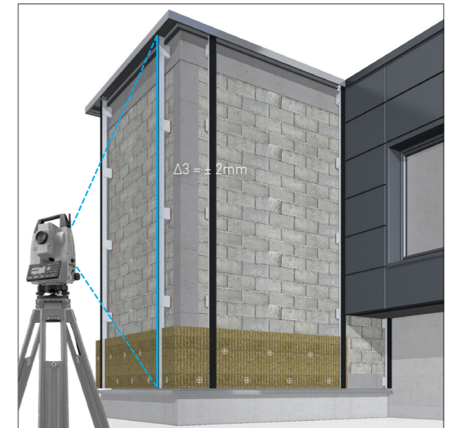
The measurement procedure for ensuring the vertical alignment of the substructure for horizontal installation.
