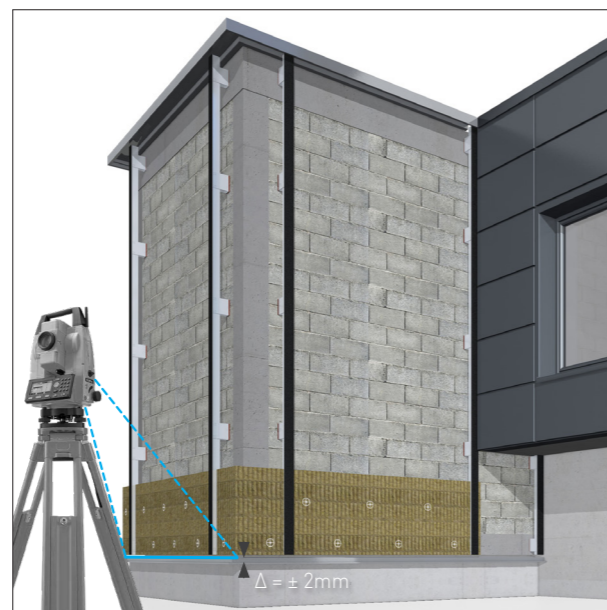
The measurement procedure for ensuring the horizontal alignment of the base support.
